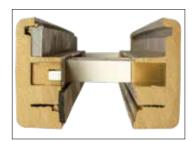
ELITE WHITE FRAME - This is our Standard Maintenance Free White Frame (Does not require painting). Specifications are: **Construction - Injected Moulded Low Profile** Surface - Woodgrain Material - White Polypropylene or White PVC Glazing Material - White foam adhesive on both channels (frame to glass & frame to door) or rubber gasket (PVC) Plugs - Used to cover screw holes Note: 18420V has a raised profile.
